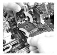
7. Visually inspect if the CPU is seated well into the socket. If not, take out the CPU with pure vertical motion and reinstall.
